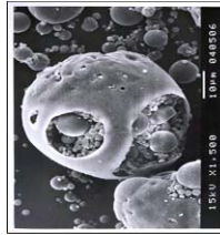
Shape of lignite fly ash magnified with electron microscope
