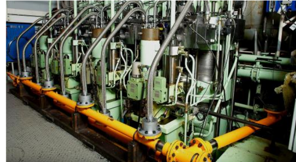
World's first low speed 2 stroke ME-GI engine Proto type
