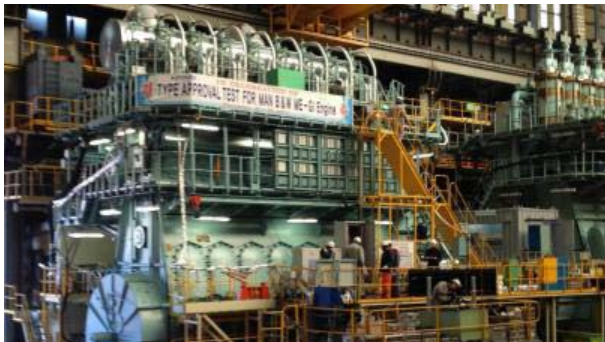
World's first commercial version ME-GI engine Type Approved by major classification societies
