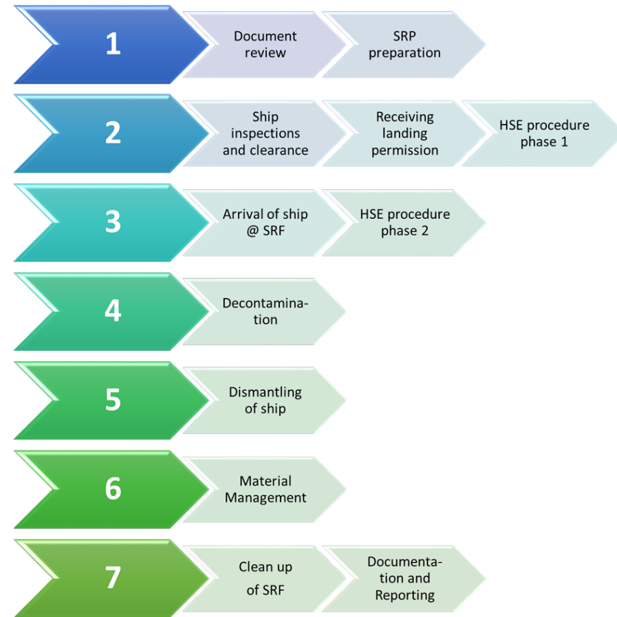
Process of ship recycling at the SRF
