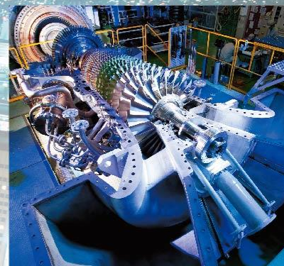
Hydrogen gas turbine
