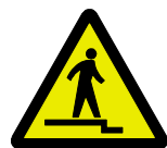
下り段差注意 Caution, uneven access/down
