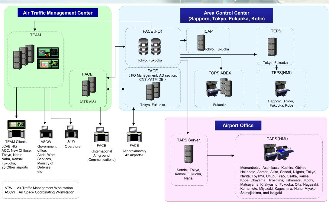
Note: The arrows in the diagram show the flow of the flight plan.
