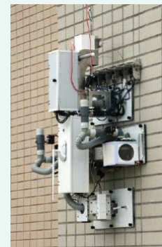
Diagram 3 Development of a device to diagnose the outside wall by attaching itself to the building wall surface and moving around Source) MLIT
