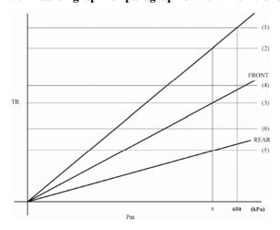
(1) =  $TR_{max}$ , when  $p_m$  = 650 kPa and supply line = 700 kPa.
