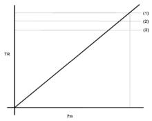
$(1) = TR_{max}$ , when  $p_m = 650$  kPa and supply line = 700 kPa.
