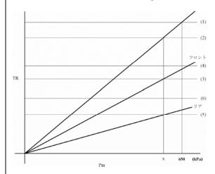
(1) = TR<sub>max</sub> (p<sub>m</sub> = 650 kPa、かつ、供給系圧 = 700 kPaのとき)
