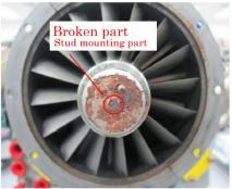
Figure 7: Corrosion on the front baring housing
