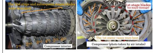
Figure 4: Compressor interior Figure 5: Leading edge of compressor
