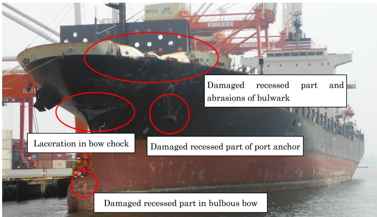
Figure 1: Damage of Vessel A (bow)
