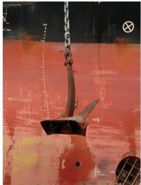
Damaged recessed port anchor shank
