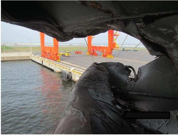
Laceration in bow chock (from the inside of fore peak tank)
