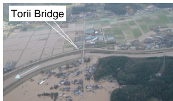
Torii Bridge Levee damage Levee breach site: around 5.4 km point on the left bank of the Izushi River
