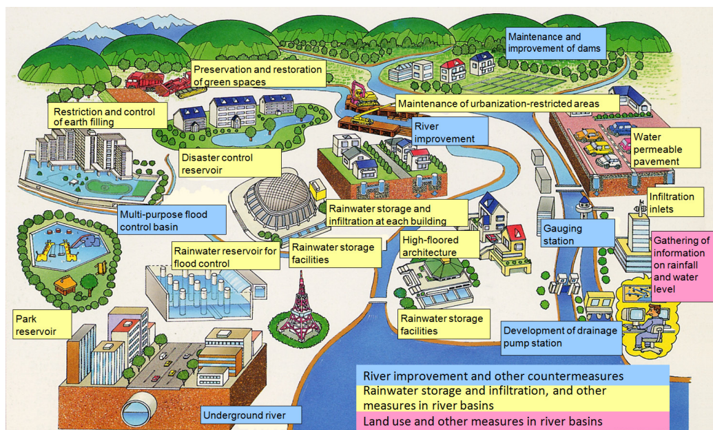
Figure3-16 Appropriate combinations of measures (Comprehensive Flood Control Measures)
