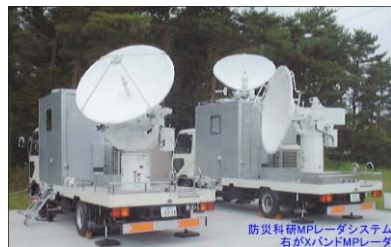
Initial development stage of MP Radar (NIED, 2000)
