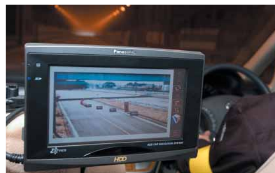
トンネル内走行中に車載器モニターへ前方の静止画像を提供 Provision of still images of road section ahead to an on-board monitor of a vehicle in a tunnel
