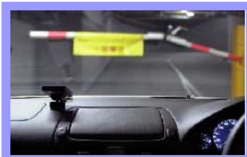
DSRC authenticates the ID number of the onboard ETC equipment
