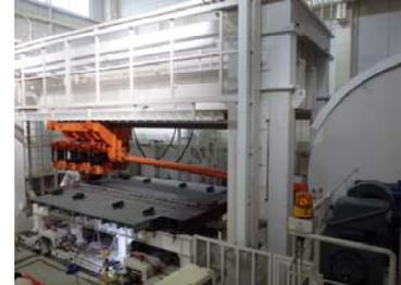
Fig. 3 Fatigue test with the wheel moving load
