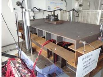
Fig. 2 Fatigue test with the non-moving loading
