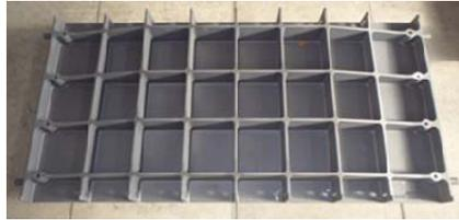
Fig. 1 Trial product of spheroidal graphite cast iron bridge
