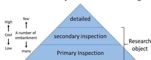
Fig 1. Process of seismic diagnosis embankment
