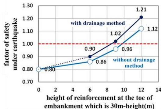
Fig 3. Relationship between the height of reinforcement and Fs
