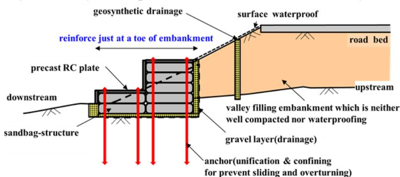
Fig 2. Aseismic reinforcement at the toe of embankment using sandbag-structure
