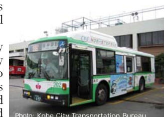
Photo: Kobe City Transportation Bureau Kobe City bus fueled by biogas generated from sewage sludge
