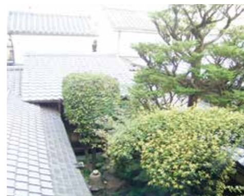
By coordinating the locations of tsubo-niwa with the neighbors, lighting and ventilation may be shared by every neighbor.
