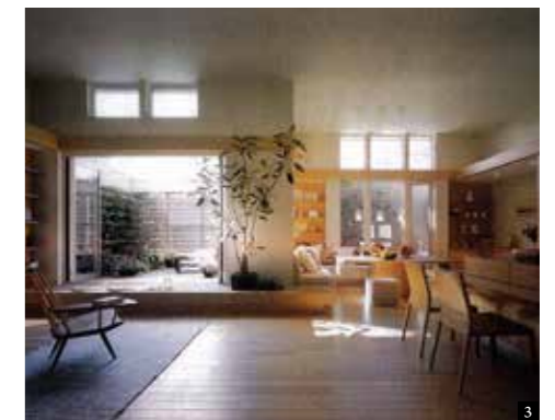
High windows mounted in the upper portion of inner opening in a room with a normal ceiling height
