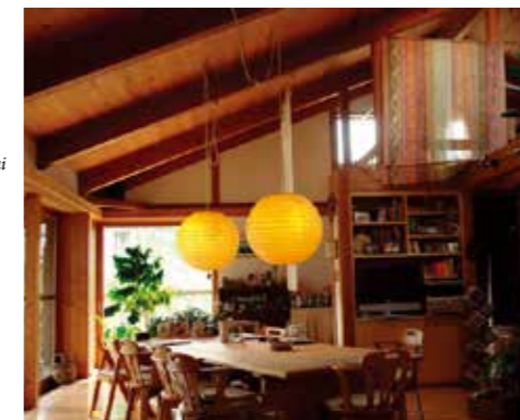
A natural house made with local wood ( Kanayama-sugi ) and other natural materials including shikkui plaster, tatami and Japanese paper.
