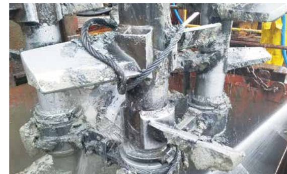
地盤改良機に巻きついた地中障害物の例／Underground obstacle wrapped around the ground improvement device
