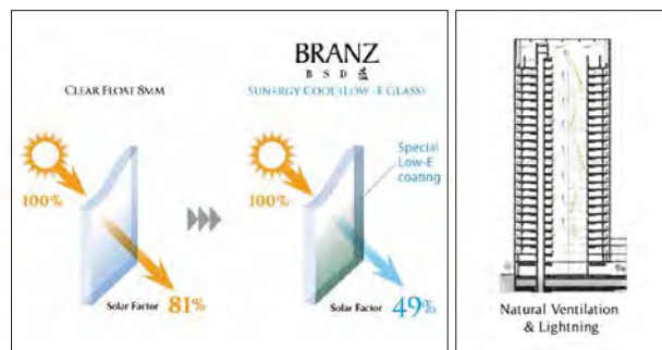
遮熱性能の高いLow Eガラス／Low-E glass with high heat shielding performance
