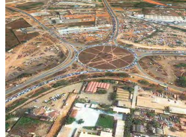
着工前のテマ交差点の様子：交通容量不足で慢性的な交通渋滞が発生／ Tema Intersection before construction: Insufficient traffic capacity causes chronic traffic congestion
