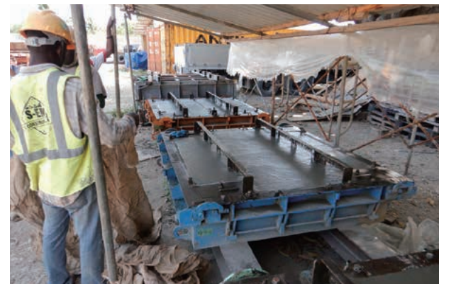
壁面材の製作状況 建材の現地製作を通じた技術移転・人材育成／ Wall surface material Terre Armee On-site fabrication: Technology transfer and capacity building through local production of construction materials
