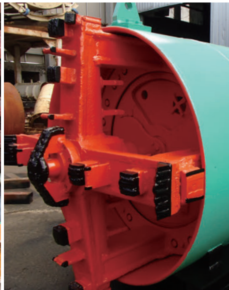
Tunnel boring machine (TBM) used for Package G construction project. TBM is set up in front of sewer pipe to excavate the ground and lead the pipes.
