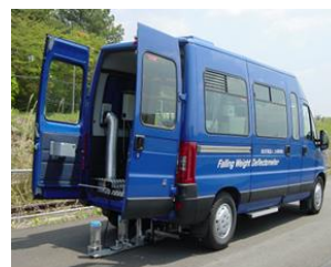
図-1 FWD (Falling Weight Deflectometer)
