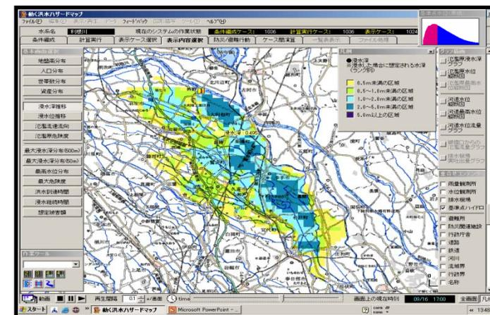
Overflow forecasting based on real time simulation
