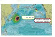
For the navigation, the weather routing technology is utilized to analyze weather information, and to provide the optimum shipping rout, taking into account the features of each ship.
