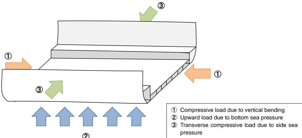
Figure A2-1 Load acting on Double Bottom Construction of Container Ships
