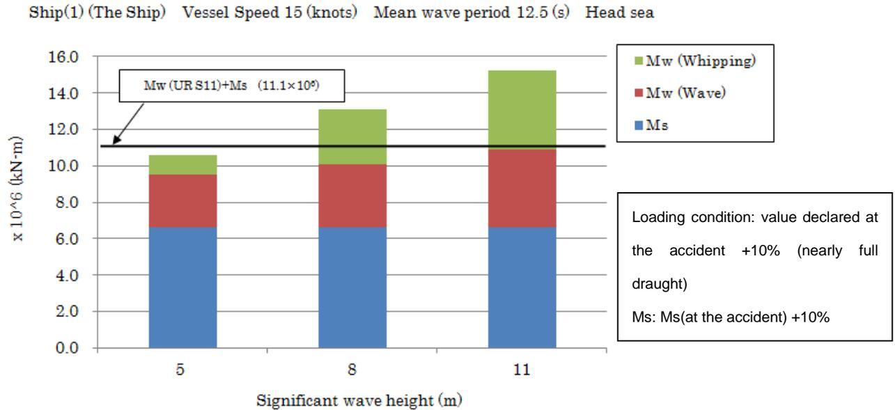
Figure 4.3.3 Relation to acting loads in IACS Unified Requirements ( $M_w(\text{URS11})$ )
