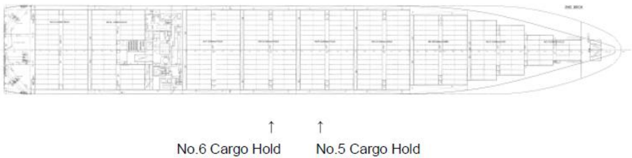
Fig 1.3.2 2 nd Deck Arrangement
