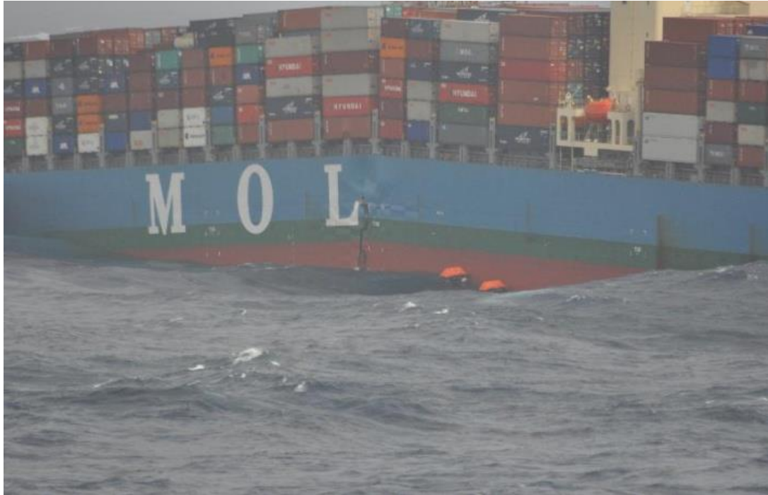
Fig 1.3.1 Condition of The Ship at the time of the accident (Direction of the crack progression (photo by Mitsui O.S.K. Lines, Ltd))
