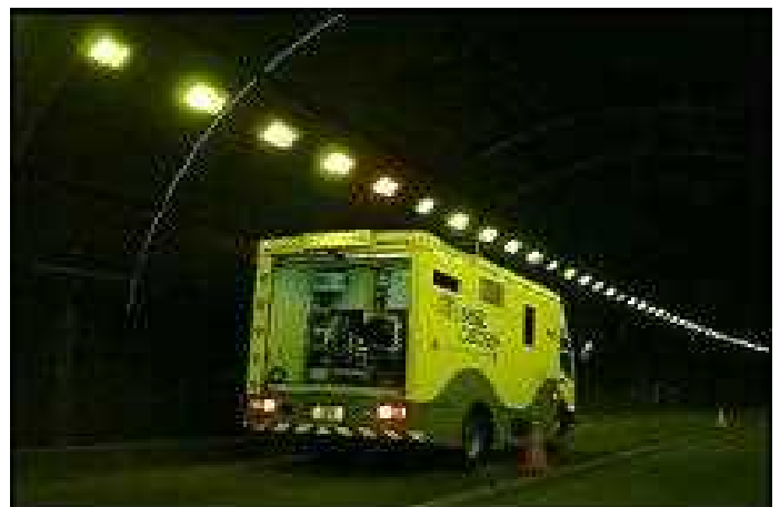
Tunnel inspection using High-Speed Concrete-crack Measurement Vehicle
