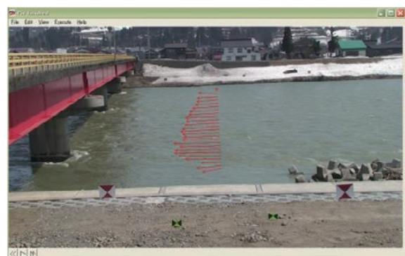
Diagram 1 Measuring the Water Level and Flow Rate Using Image Analysis of Video Source) Fujita Lab, Kobe University Faculty of Engineering
