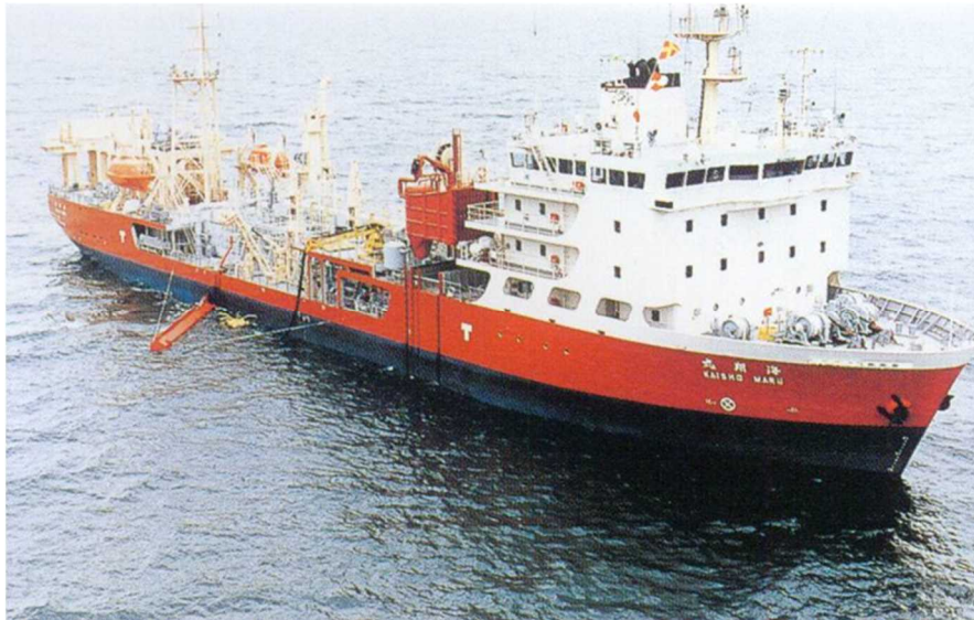
Figure 29. Trailing Suction Hopper Dredger with Oil Recovery system “Kaishomaru”
