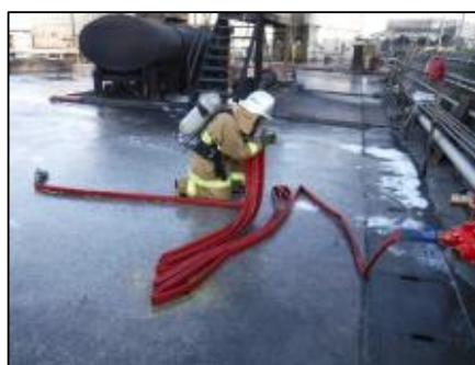
Step 4 Prepare for extending fire hoses. (The photo shows preparing the hose by the coil method)
