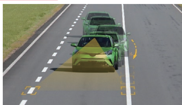
Figure II-7-4-11 Lane departure prevention system
