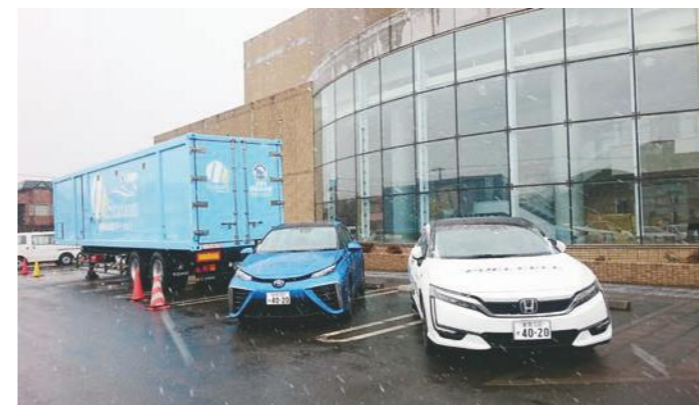
Mobile hydrogen station and fuel cell vehicles
