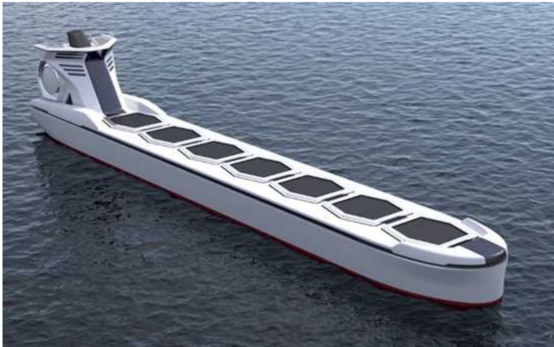
Figure Appendix 3.1-5: Bird's Eye View of the Hydrogen-fueled 80,000 DWT Bulk Carrier
