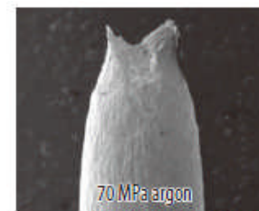
70 MPa argon Impact of hydrogen on metals undergoing tensile testing
