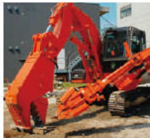
Robot separating waste material at a construction site
