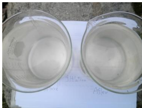
Treated water with no change in turbidity (left: raw water before filtration; right: treated water after filtration)
