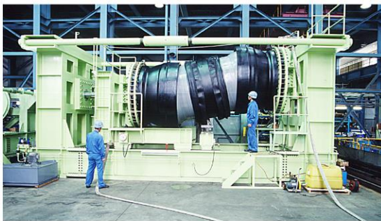
Inspecting water tightness of the world largest TAI-FLEX DN 1800mm of subsiding
