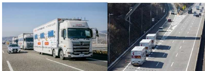
Figure 1-2-9 Truck platooning traveling on the Shin-Tomei Expressway
