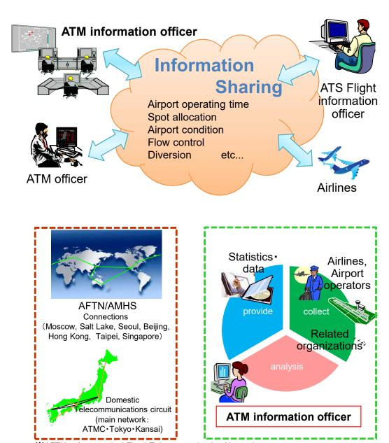
※AFTN : Aeronautical Fixed Telecommunication Network AMHS: ATS(Air Traffic Service) Message Handling System
