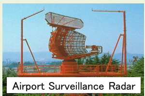
Airport Surveillance Radar Detects positions of flying aircraft
