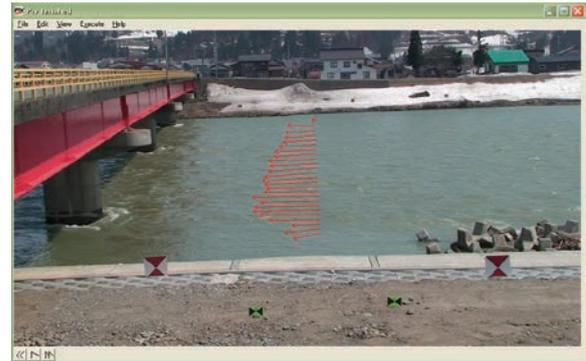
Diagram 1 Measuring the Water Level and Flow Rate Using Image Analysis of Video
