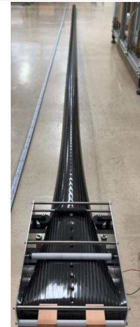
Extension test of 10m length CFRP bistable boom
