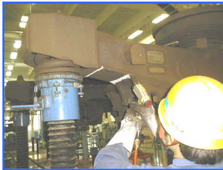
Stripping operations for areas of bogie frame to be inspected
