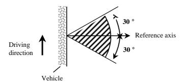
With regard to the range of visibility angles in right-and-left direction, the figure shows the device mounted on the right side.
