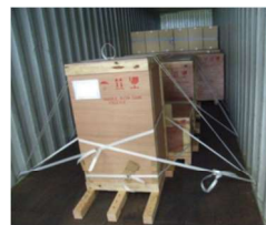
Figure 30 Securing examples using cord straps
