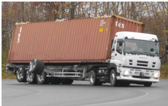
Figure 7 Trailer at rollover limit
