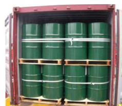
Figure 30 Securing examples using cord straps
