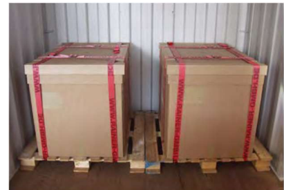
Lashing with a combination of pallets and straps
