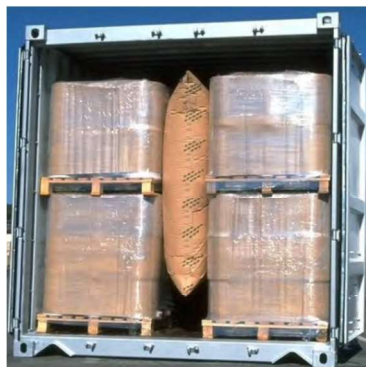
Securing cargo using airbags for dunnage
