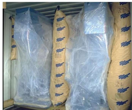
Securing cargo using airbags for dunnage
