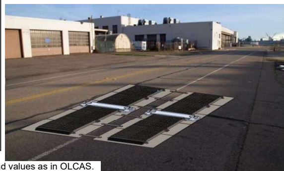
Figure 45 Image of road-mounted measuring instrument (from All Nippon Checkers Corporation / Mitsubishi Nagasaki Machinery Mfg. Co., Ltd.)
