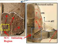
The aft fractured surface was caused by SCC initiated by the corrosion generated on the lubrication passage, which then led to progressing cracking due to repetitively imposed loads.
