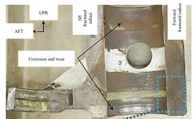
The forward fractured surface had an initiating region of corrosion on the lower side of the pivot boree, then was generating SCC and finally was fractured due to repetitively imposed loads.
