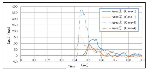
Analysis of Time Series of Vertical Impact Force on the bottom of the ship
