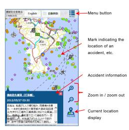
Screen showing the information of current location using GPS function
