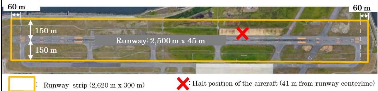
Figure 2 Runway strip of runway 10/28 at Niigata Airport (aerial photograph of Google Earth with some explanatory modifications added)
