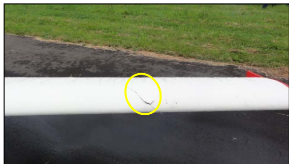
Cracked left wing
