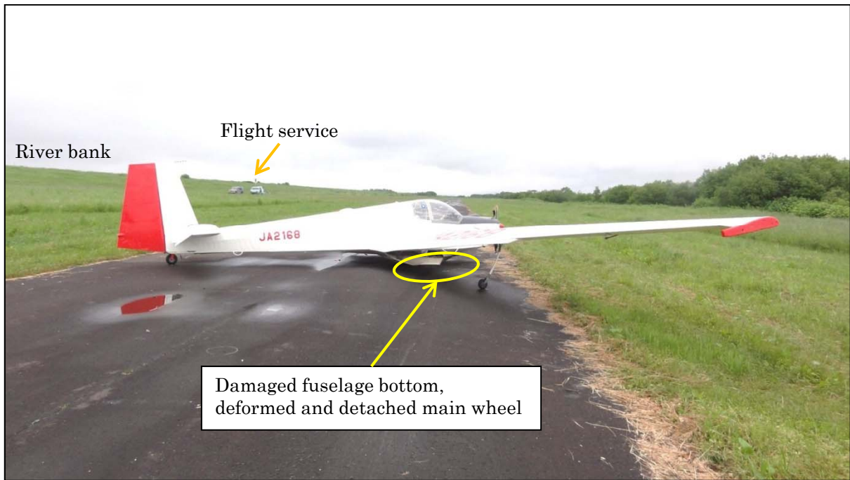
Deformed and detached main wheel
