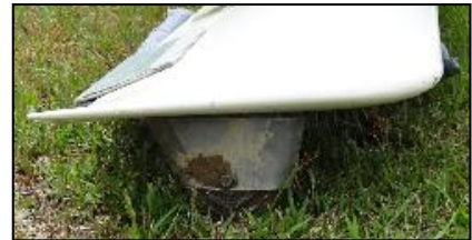
Figure 5: Auxiliary wheel at the right wing tip
