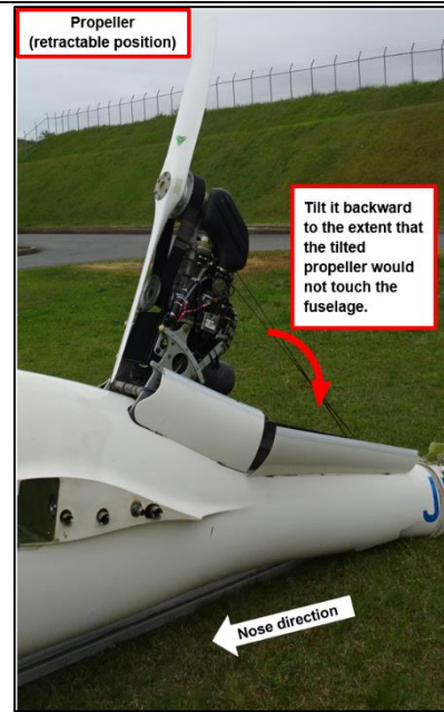
Figure 2: Appearance of the extended engine
