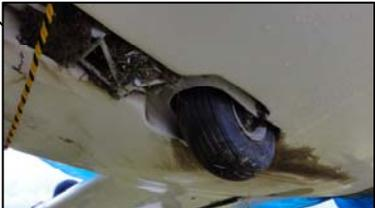
The locking device of the nose landing gear was damaged and the gear was pushed back
