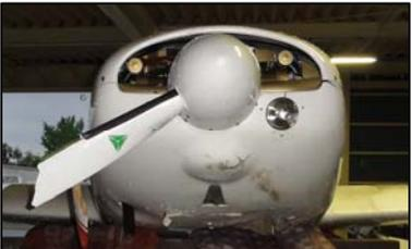
Front (Broken propeller, cracks in the lower side)
