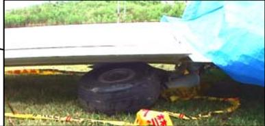
Left main landing gear was broken outward (taken from the rear of the left main landing gear)
